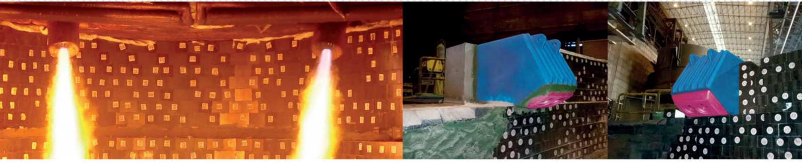
The TEKNOSPHERA has been designed to contain and protect the lance with the possibility to change the inclination in the EBT zone. The TEKNOSPHERA is made up of 100% copper fusion with internal canals in which the water circulates.
