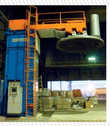
The VERTICAL LADLE HEATER consists of a base fixed to the ground, over which rotates an arm that supports the ladle heater with the burner in the center.
