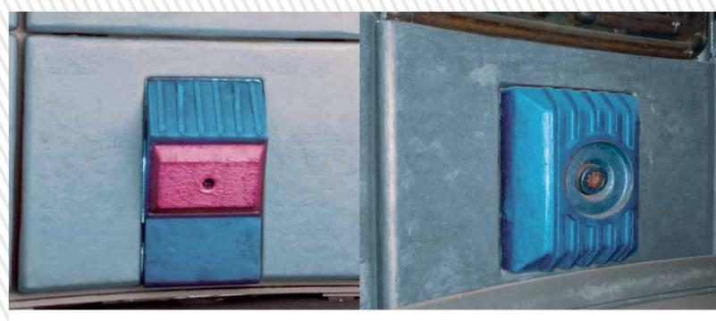
The BURNER BOX has been designed to contain and protect the burner in the EAF. It is 100% monolithic casted copper component without welding with internal canals of rectangular cross-section in which the water circulates.
