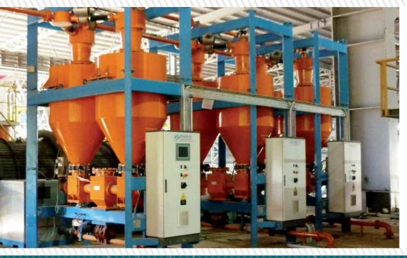
The BIROCH can mix carbon and lime together. It also allows to grind, mix and inject the following powders: refractory bricks, electrode remains. The injection allows the transportation of the material with air generated at a temperature of about 120°C at high flowrate and low pressure. The maximum flow is of 200kg/min.
